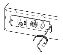
Be sure to fully tighten the screws. If they are loose, the ground connection between the board and the T-4555 may be inadequate, resulting in noise or failure.
